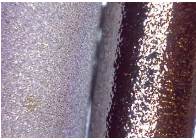
Close up of two tubes before (left) and after electropolishing. Short-wavelength roughness is strongly reduced, while long-wavelength roughness largely remains
