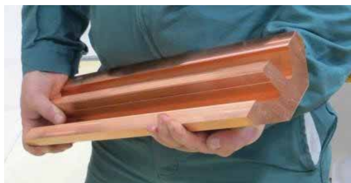
A major vane of the compact high-frequency RFQ, illustrating its compactness
