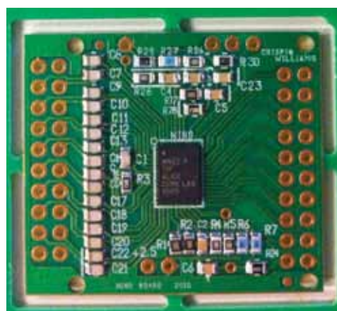
A printed-circuit carrier board for the NINO chip
