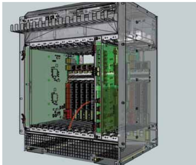
View of a full-size 14-slot SRS-ATCA crate
